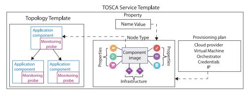
Fig. 5. The TOSCA orchestration standard with its templates, application and provisioning plan description as they are mapped to TOSCA and used in the SWITCH workbench.
