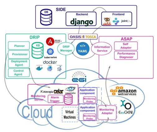
Fig. 2. Overall architecture of SWITCH. The main components of the system, SIDE, DRIP and ASAP are colour-coded. Technologies used are identified by their icons or logos. (For interpretation of the references to colour in this figure legend, the reader is referred to the web version of this article.)
