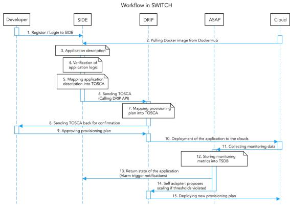
Fig. 7. The sequence diagram presents workflow in SWITCH workbench among all three subsystems (SIDE, DRIP, ASAP).
