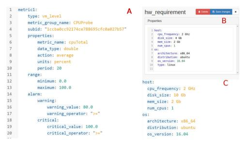
**Fig. 6.** An example of TOSCA containing the Alarm trigger definition (A), an example of UI describing hardware requirements (B), and the corresponding entry in TOSCA (under TOSCA $\rightarrow$  Node template $\rightarrow$  Constraints (C)).
