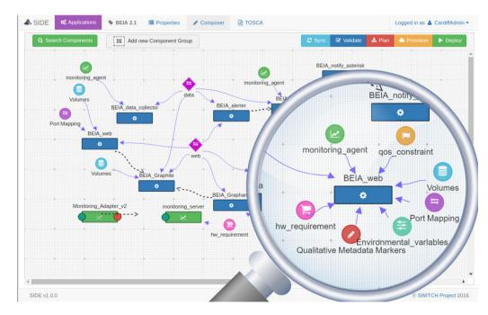
Fig. 3. Example of an application composition in the SWITCH workbench. In the magnifying glass all properties that can be linked to the component and set as constraints are shown. The entire modelling graph presents the application composition of the BEIA use case. It is made up of various components to which properties are attached. (For interpretation of the references to colour in this figure legend, the reader is referred to the web version of this article.)
