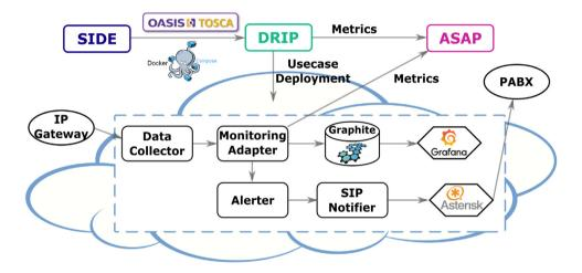
Fig. 9. Functional diagram for an elastic disaster early warning system.
