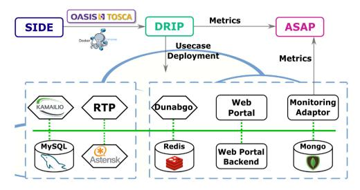
Fig. 8. Architecture of the real-time UC platform.
