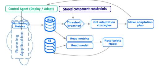
Fig. 4. The dataflow of an ASAP adaptation solution.
